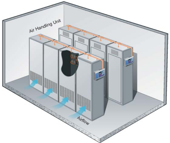
Fig 4. In-Cabinet Capillary Sampling for Switch Rooms
